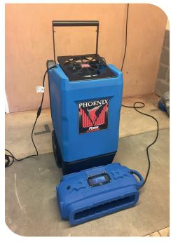
Boost Bar adds controlled heat to the process air of many drying system.
