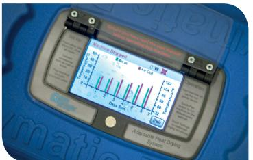
Boost Bar continuosly monitors and logs energy usage and temperature differential across the heater.
