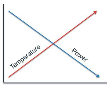
Boost Bar adjusts its power consumption based on the volume of incoming airflow and also the temperature of the incoming airflow. If airflow is lost the Boost Bar automatically powers down the heating elements and waits for airflow to return.
